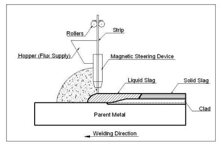
From last many decades CRA (Corrosion resistant alloys) are being used for overlaying a protective layer over base metal by various techniques like explosion welding, SAW, Submerged arc Strip Cladding (SASC) and Electro-Slag Strip Cladding.The most efficient and widely used technique these days is Electro-Slag Strip cladding due to its unique properties like high deposition rate, Low dilution and high quality defect free weld.
